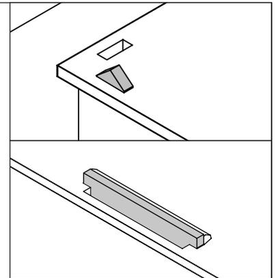
**7** Insert tabs on Drop Tile into slots on Back Panel
