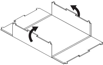
**6** Insert tabs on Drop Tile into slots on Back Panel
