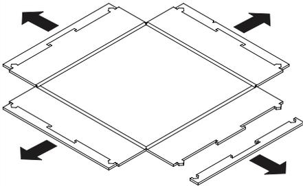
**2** Orient Drop Tile with v-cuts facing upward
